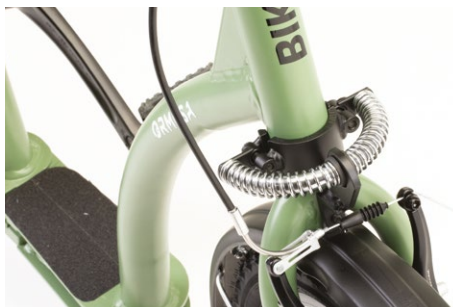
882 Steering limiter with spring.
