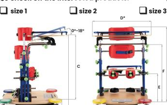
\*in size 1 the greatest encumbrance is given by the table. In sizes 2 and 3 it is given by the knobs.
