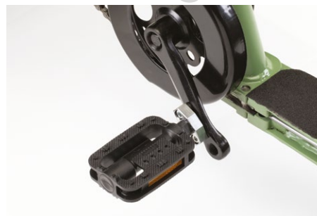
847 Cranks adjustable in length
